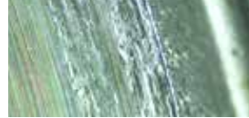
Bare metallic clamping nut after 15 clamping cycles
